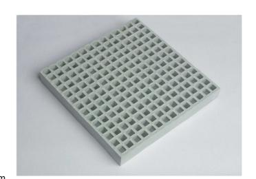
The GRP gratings are according to the rules of the Accident Prevention & Insurance Association Germany and the DIN 24537-3 gratings as floor covering Part 3: GRP gratings, walkable up to distance between supports of 550 mm. Necessary supports are set by the customer!
