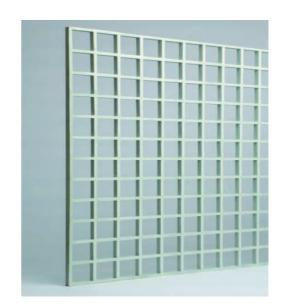
The GRP gratings are according to the rules of the Accident Prevention & Insurance Association Germany and the DIN 24537-3 gratings as floor covering Part 3: GRP gratings, walkable up to distance between supports of 250 mm. Necessary supports are set by the customer!
