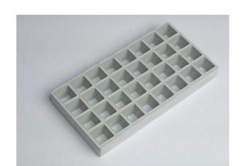
The GRP gratings are according to the rules of the Accident Prevention & Insurance Association Germany and the DIN 24537-3 gratings as floor covering Part 3: GRP gratings, walkable up to distance between supports of 710 mm. Necessary supports are set by the customer!.
