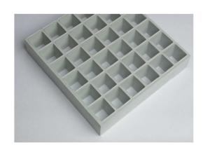
The GRP gratings are according to the rules of the Accident Prevention & Insurance Association Germany and the DIN 24537-3 gratings as floor covering Part 3: GRP gratings, walkable up to distance between supports of 850 mm. Necessaire supports are set by the customer!
